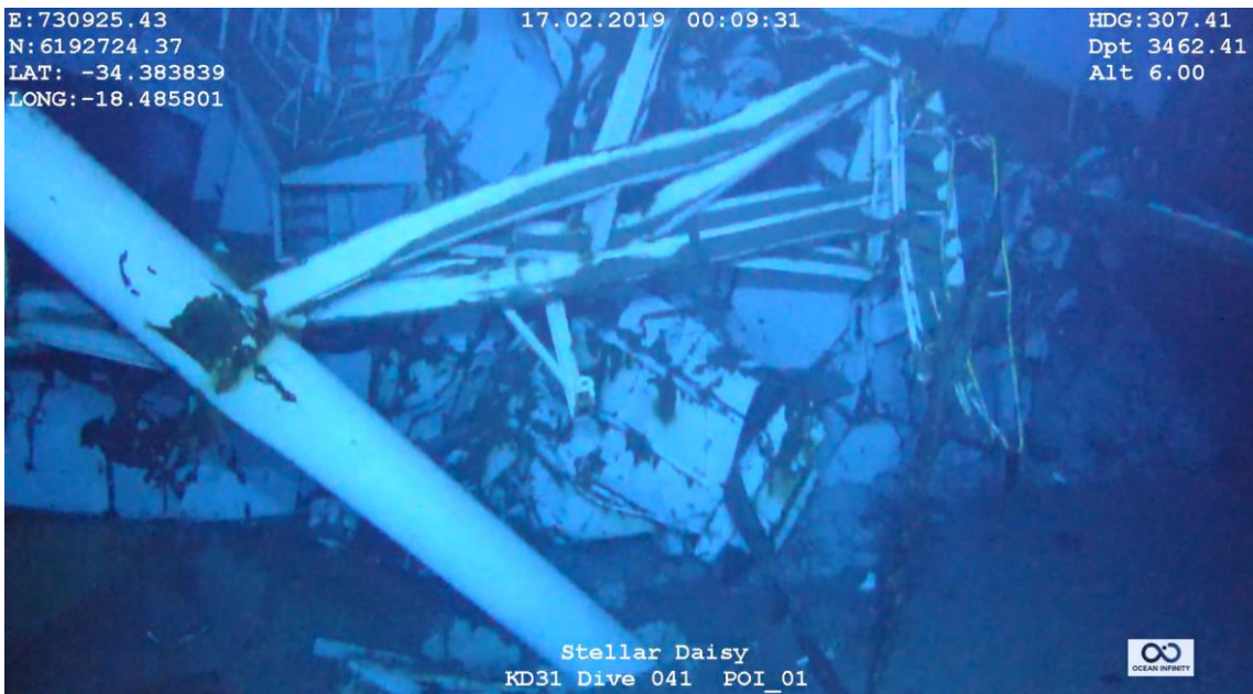
Figure 4-4; ROV image of port side of superstructure highlighting crushing of lower level(s) of the superstructure
