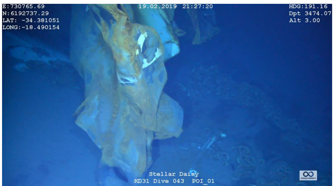
Figure 4-10; ROV video image illustrating the condition of bow section
