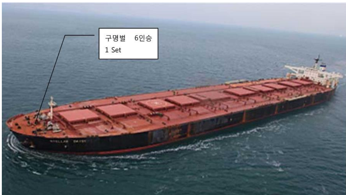
Figure 3-4; Client supplied annotated image highlighting life raft location on deck level at the bow, fore of the bow mast
