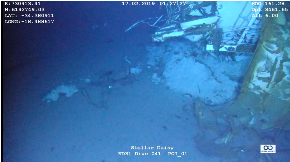
Figure 4-3; ROV image of starboard side of the superstructure highlighting burial of lower structure in the seabed / iron ore material
